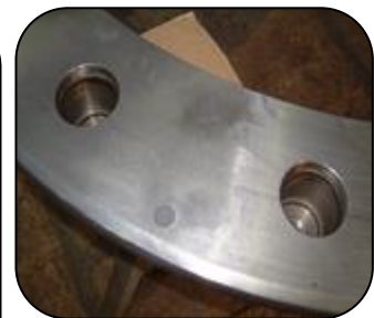
Turbine cover repaired using PES 107 Power Metal Repair Paste XL
