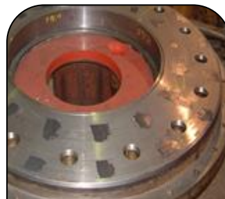
Turbine cover repaired using PES 107 Power Metal Repair Paste XL
