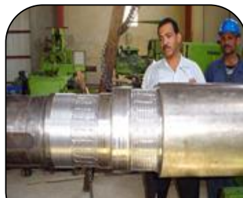
Quarry crusher shaft rebuilt using PES 107 Power Metal Repair Paste XL
