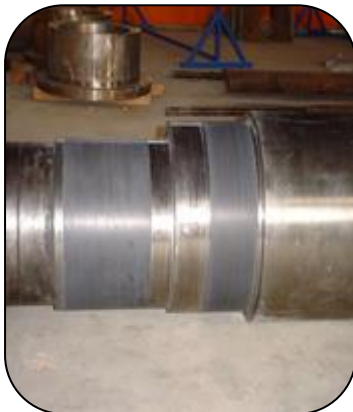
Quarry crusher shaft rebuilt using PES 107 Power Metal Repair Paste XL
