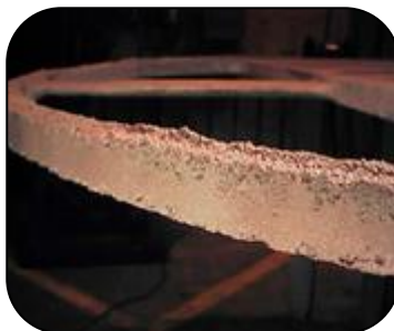
Quarry crusher shaft rebuilt using PES 107 Power Metal Repair Paste XL
