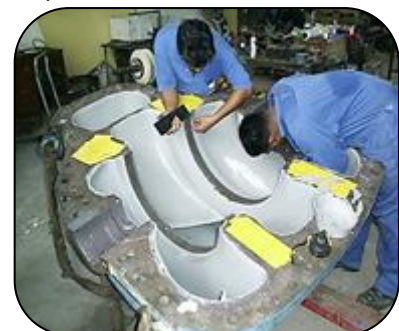
Process vessel surfaces badly corroded from chemical attack rebuilt using PES 201 Ceramic Repair Paste
