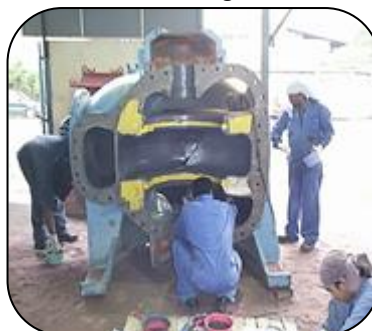
Process vessel surfaces badly corroded from chemical attack rebuilt using PES 201 Ceramic Repair Paste
