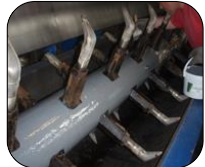
Process equipment abrasive blast cleaned and resurfaced using PES 202 Ceramic Repair Fluid
