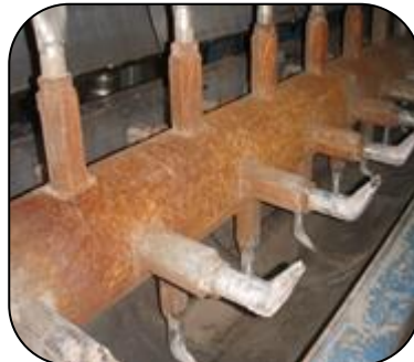
Process equipment abrasive blast cleaned and resurfaced using PES 202 Ceramic Repair Fluid
