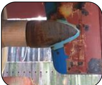
Rudders resurfaced and protected
