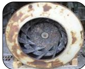
Hot air fan, abrasive blast cleaned and coated with PES 203 Super Flow
