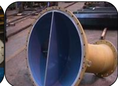
Process pipework abrasive blast cleaned and coated with PES 203 Super Flow
