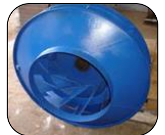
Hot air fan, abrasive blast cleaned and coated with PES 203 Super Flow
