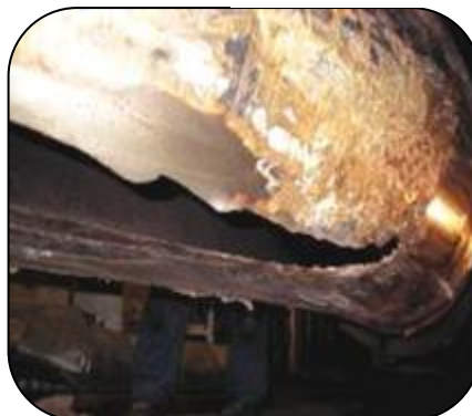
Coal grinder at a steelworks relined and repaired using 204 Heavy Duty Ceramic Repair Paste
