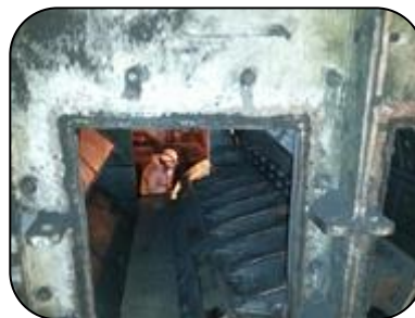
Coal grinder at a steelworks relined and repaired using 204 Heavy Duty Ceramic Repair Paste
