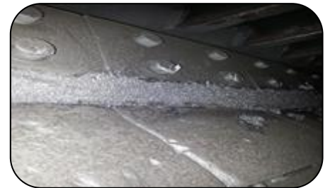
Coal grinder at a steelworks relined and repaired using 204 Heavy Duty Ceramic Repair Paste
