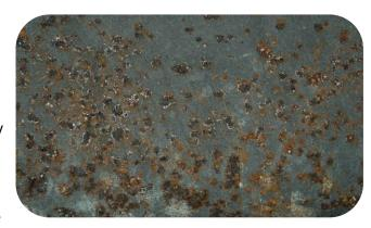
if the level of salts has been reduced sufficiently to begin coating work. It is common to have to perform this wash down process several times to achieve the required surface cleanliness.
