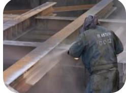
We recommend for the best profile that angular grit of 80-12 mesh size grain be used To achieve a surface profile of the steel ranging from 3-4 mils.
